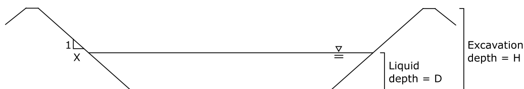
Figure 13. Profile view of typical manure storage lagoon construction. Not drawn to scale; the vertical scale on this diagram is exaggerated to show the side slopes and liquid level clearly.
